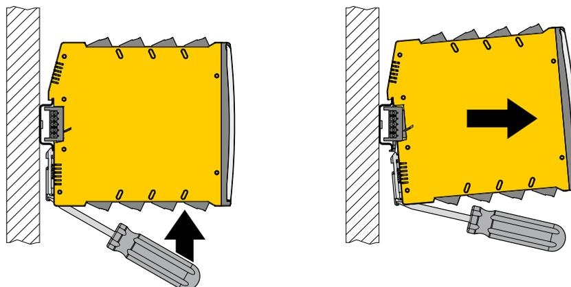
Fig. 4: Remove device
