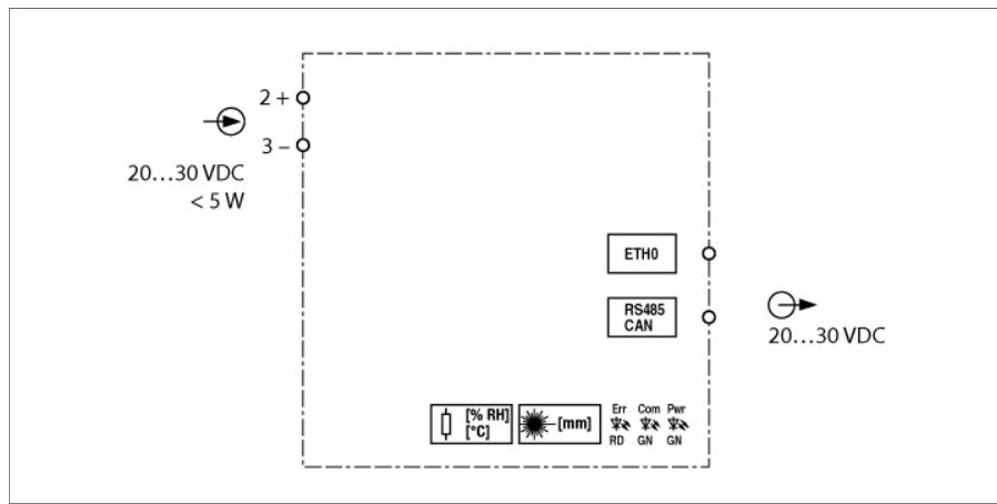
The cabinet guard IM18-CCM40-MTI/24VDC uses integrated sensors to monitor temperature, relative humidity and the distance from the control cabinet door. For example, the information can be transferred to higher-level systems via the Ethernet interface.
