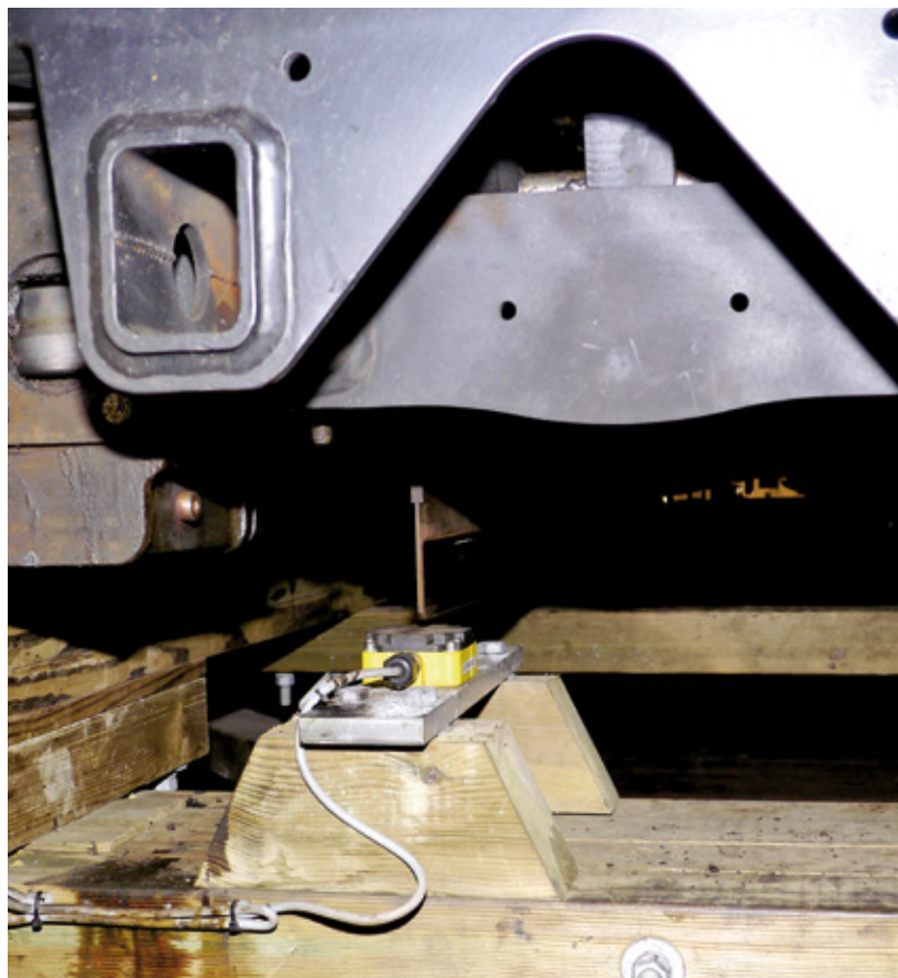
The view below the train shows the copper brake fin of the Wodan Timbur Coaster carriage above the robust uprox+ sensor
