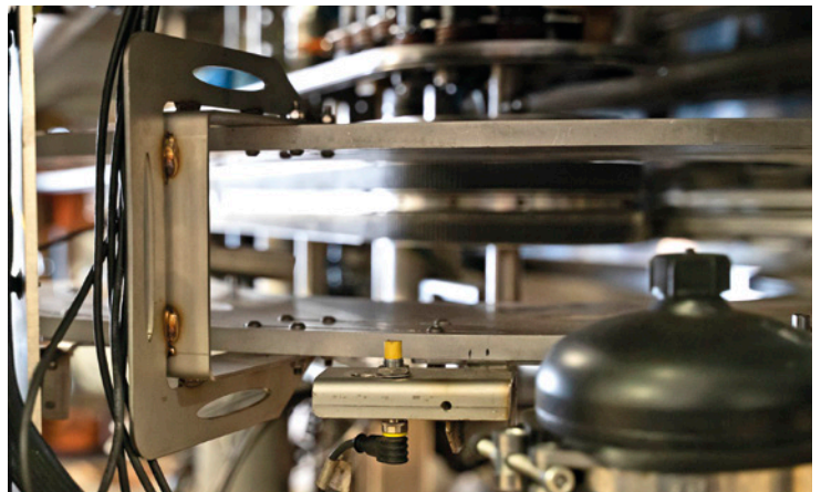
Inspector with large detection range: When a cassette passes the NI10U-M12 proximity switch, the PLC starts the timer for a harvesting operation
