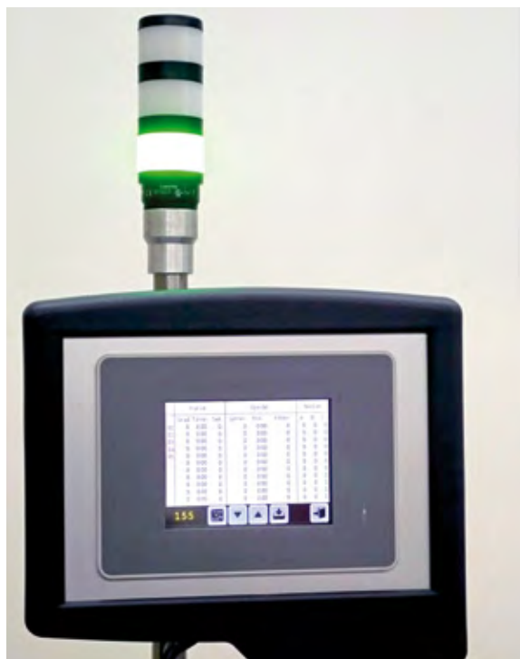
The core of the "new" machine is Turck's VT250 HMI/PLC, programmable with Codesys 3
