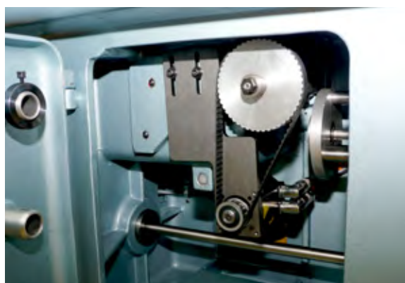
There is still a lot of space in the gear box after the servo motors have been installed
