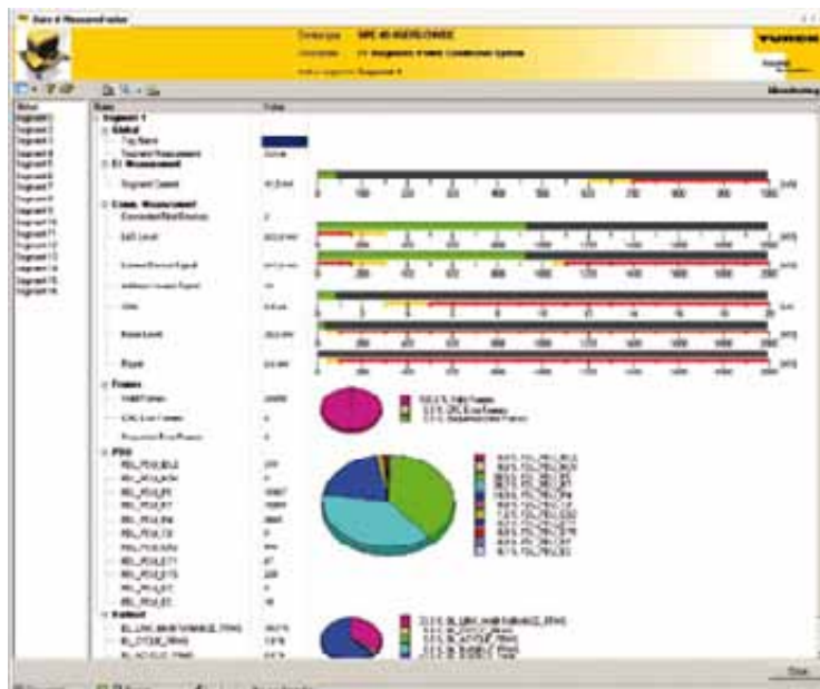
The DPC system continuously monitors the entire periphery and displays faults such as voltage drop or temperature drift
