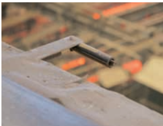
Reference points: The RFID tags are mounted on specified positions of the crane's travel path
