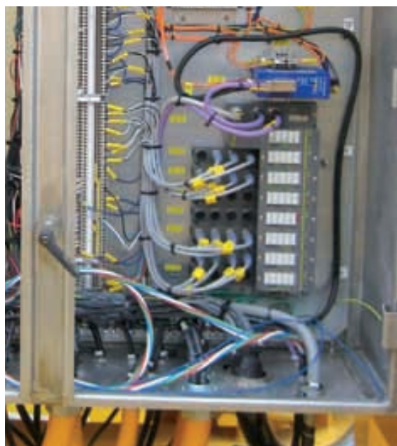
Tough: Turck's BL67 remote I/O system can take the impacts and vibrations from the gantry cranes
