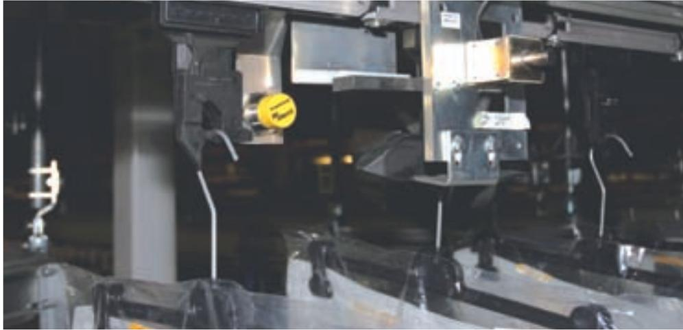
The data carriers, with a diameter of 20 mm, are integrated in the transport slide
