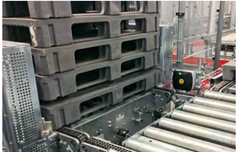
The plastic pallets come ex-factory with a UHF tag
